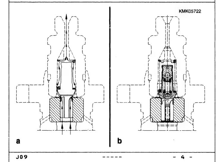
At the end of injection, the pressure drops off on the pump end and the GDV closes.
